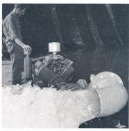
60.5-hp V-4 on 3000 gpm pump
