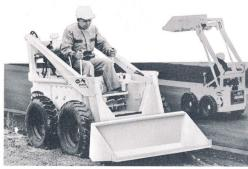
25-hp VF4D powering front-end loader
