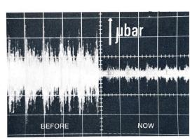
Before and after noise level graph for valve gear train.
